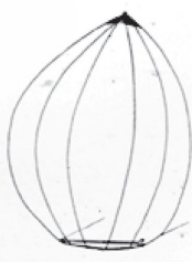
Figure 5. A parachute spinnaker, showing how it will fill and spread though only a small boom is used
