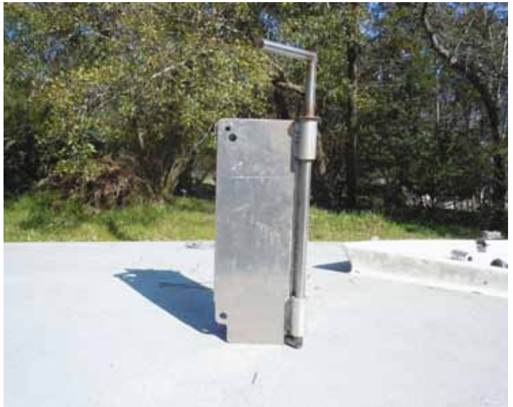
Side view of housing that captures bottom of mast. Stainless bar is spring loaded stop that keeps mast footed. Hole at bottom left fits to deck pivot, top left hole is for bolt that retains mast in housing.
