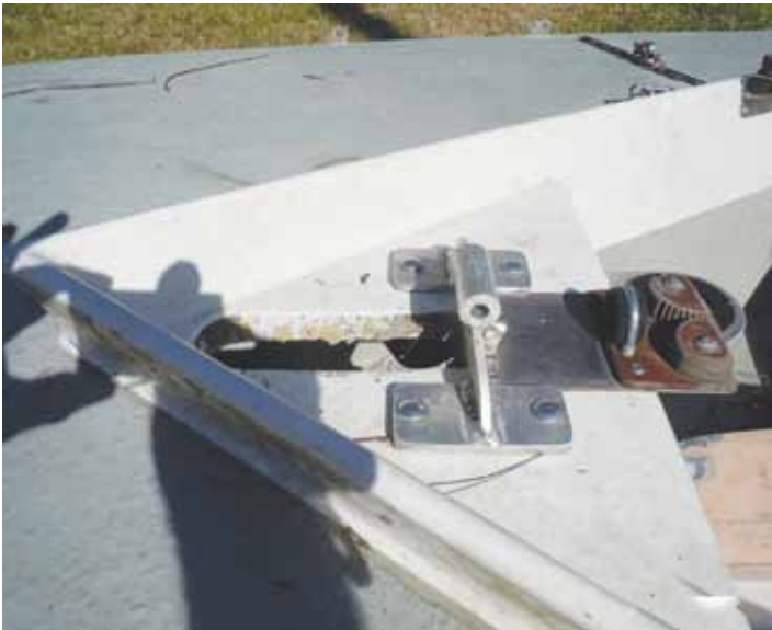
Permanent pivot mounted at mast opening. Doubles as vang purchase but could be demountable using recessed threaded fittings.
