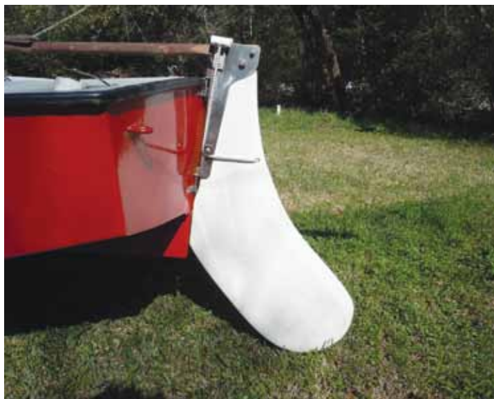
Rudder is captured in stainless steel housing and is retained with bungee chords. Cords go through rudder, back to rollers and up to eared retainers.
