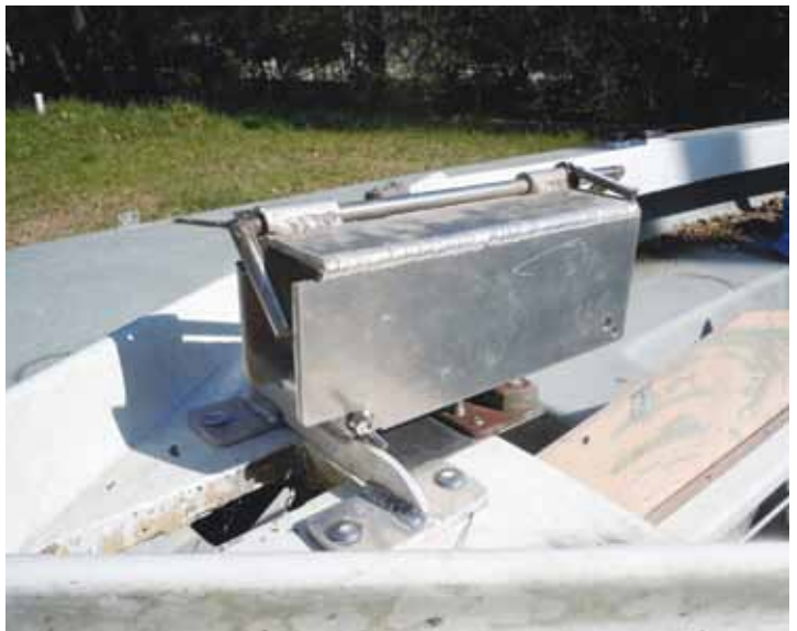
View with pivot bolt in place and ready to receive mast. Note stopper rod location.
