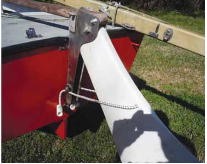
View with bungees released. Note ears at top of housing and rollers near bottom of housing.
