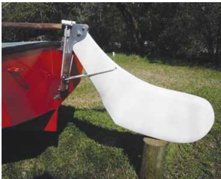
Rudder in kick up mode with bungees in tension.
