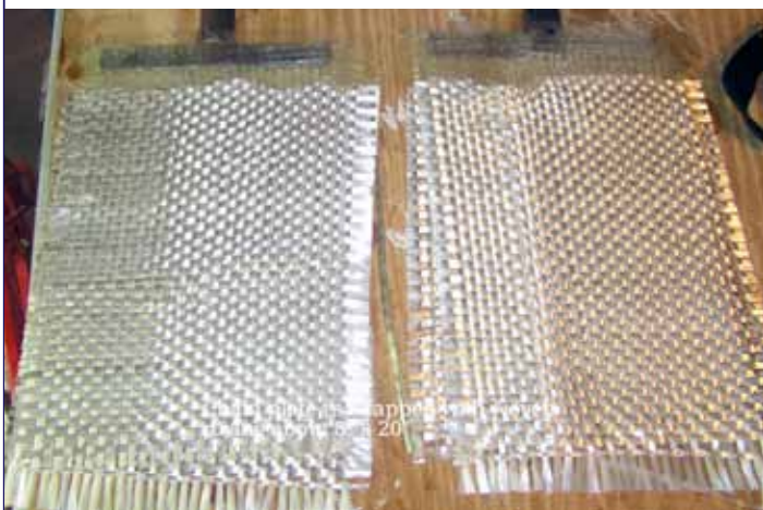
Chainplate tees wrapped with woven roving prior to bonding to the hull. Only pre-epoxy the "Tee" part of the chainplate. Not more as I have done. This pre-epoxying was done to be certain that the roving fitted snugly around the Tee. Tension was applied to the chainplate/glass to aid in the snug fit. The overall size of the plate wrap was 8" wide and length to fill the cut out area with the chainplate in the installed position.
