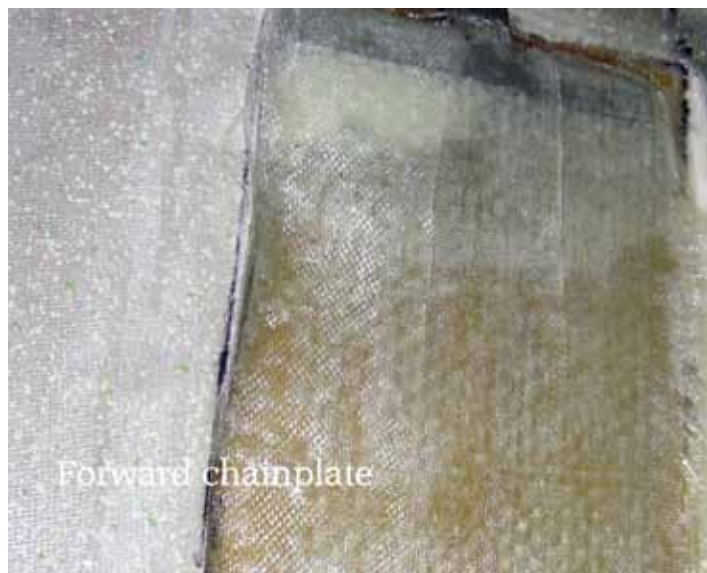
Forward chainplate epoxy bonded to hull with 3" wide fiberglass tape layered over woven roving. It may not look like total wet out has been achieved but it was. Tape was used to cover the woven roving because it has a woven selvege and does not unravel so everything will be neater.
