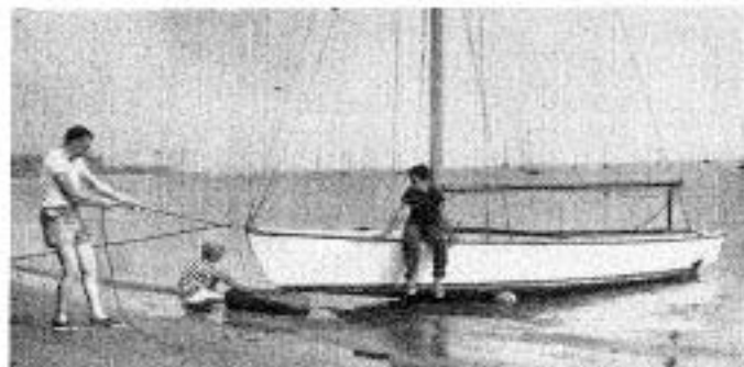
The boat's weight is being carried by one Airoller while the second one is placed under the bow. Two Airollers are required for a Lightning—with three the job is somewhat easier.
