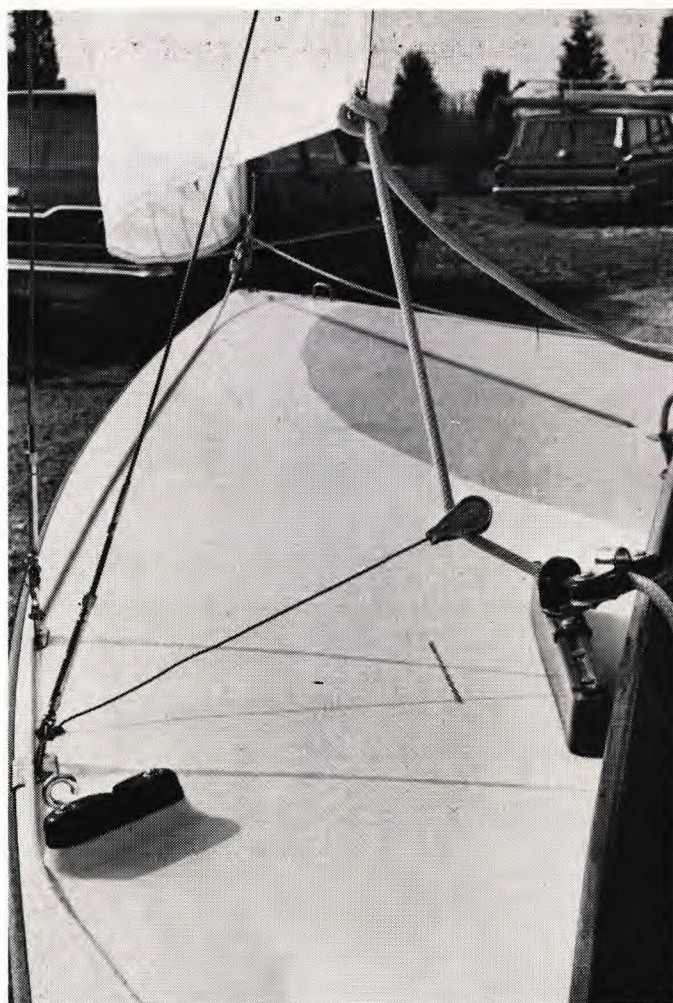
5. Single jib sheet rig with Barber hauler. The painted line on deck denotes 13 degree angle. Note spinnaker guy cleat. Jib tack should be down closer to deck.
