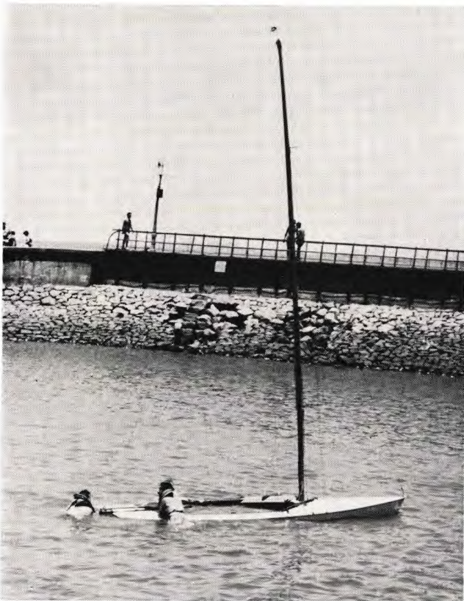
Boat upright by standing on centerboard—crew on each side to prevent roll.
