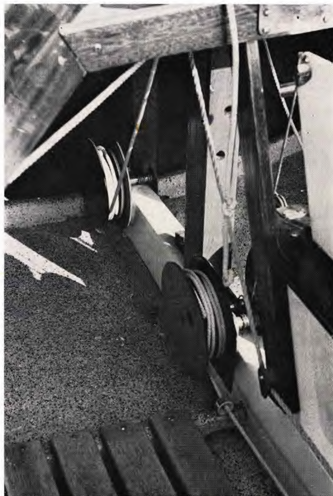
3. Drum winches for the jib downhaul, boom vang, and centerboard.
