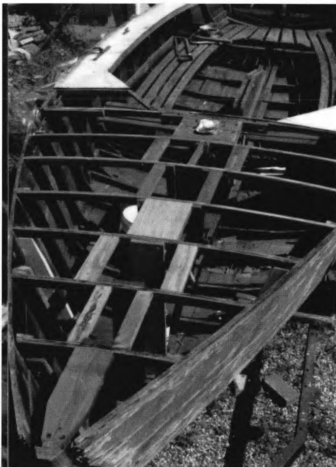
Restoration in very early stage - new stem is installed.
