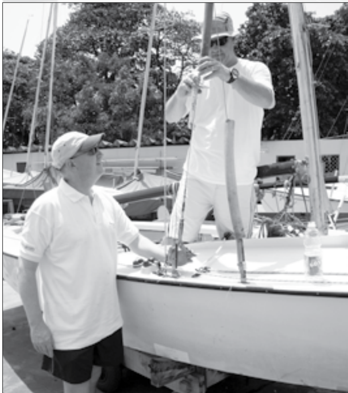
Note: the lever adjustment to relax the shrouds
